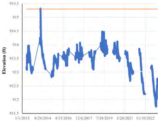
Figure A-3: Water surface elevation on Duck Lake from 2013 to 2023 & Ordinary High-Water Level (915.3 ft).
