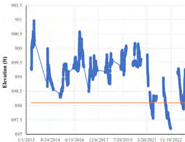
Figure A-23: Water surface elevation on Silver Lake from 2013 to 2023 & Ordinary High-Water Level (898.1 ft).
