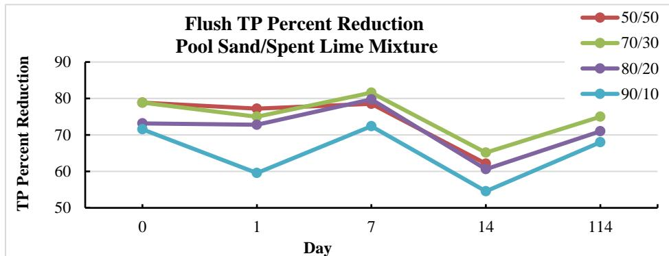
**Figure 4-37 Pool Sand/Spent Lime Mixture Column Testing Phosphorus Removals**
