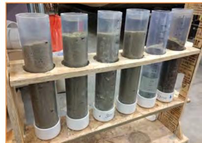
Figure 4-36 Spent Lime/Sand Mixture Column Testing
