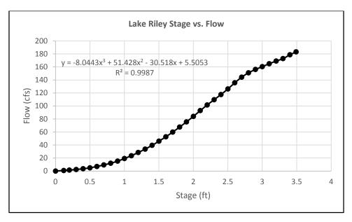
Figure B.3 Relationship between stage and outflow
