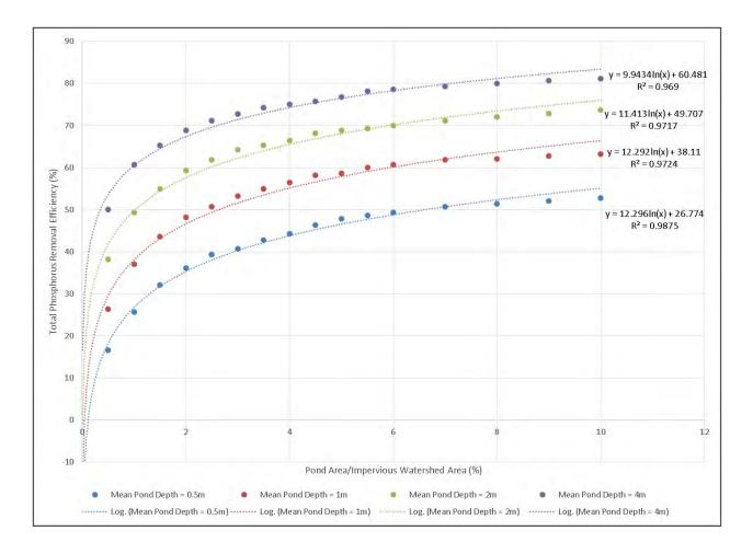
Figure A.1 Curves relating detention pond surface area, watershed impervious area, pond depth, and total phosphorus removal efficiency
