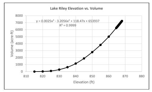
Figure B.1 Relationship between lake volume and elevation
