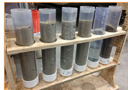
Figure 4-31 Spent Lime/Sand Mixture Column Testing
