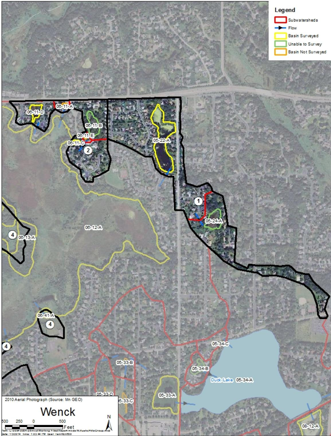
**Figure 3.3. Constructed Ponds, Wetlands and Flow Patterns in the North Rustic Hills Park Area Subwatershed.**
