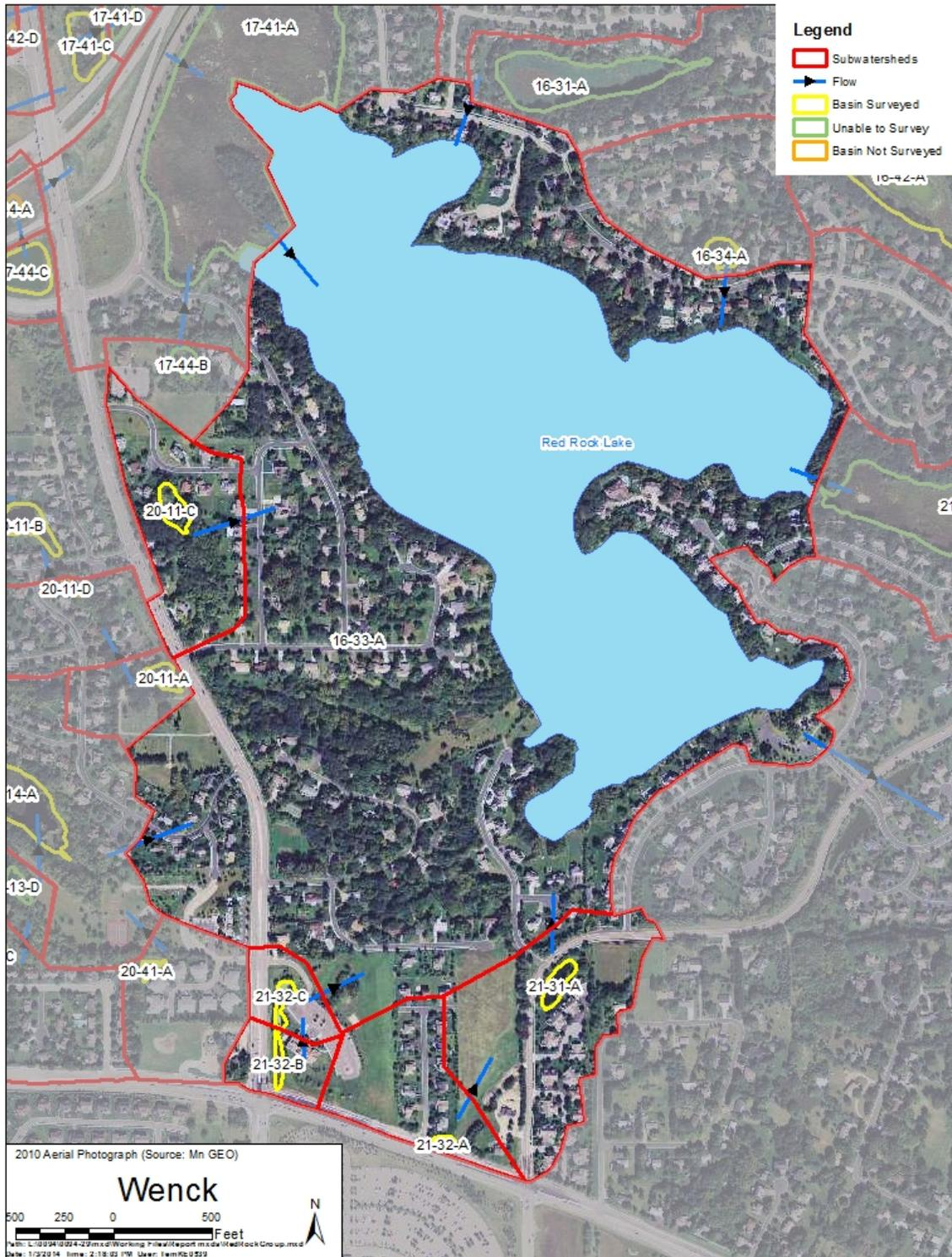
**Figure 3.10. Constructed Ponds, Wetlands and Flow Patterns in the South Red Rock Lake Area Subwatershed.**
