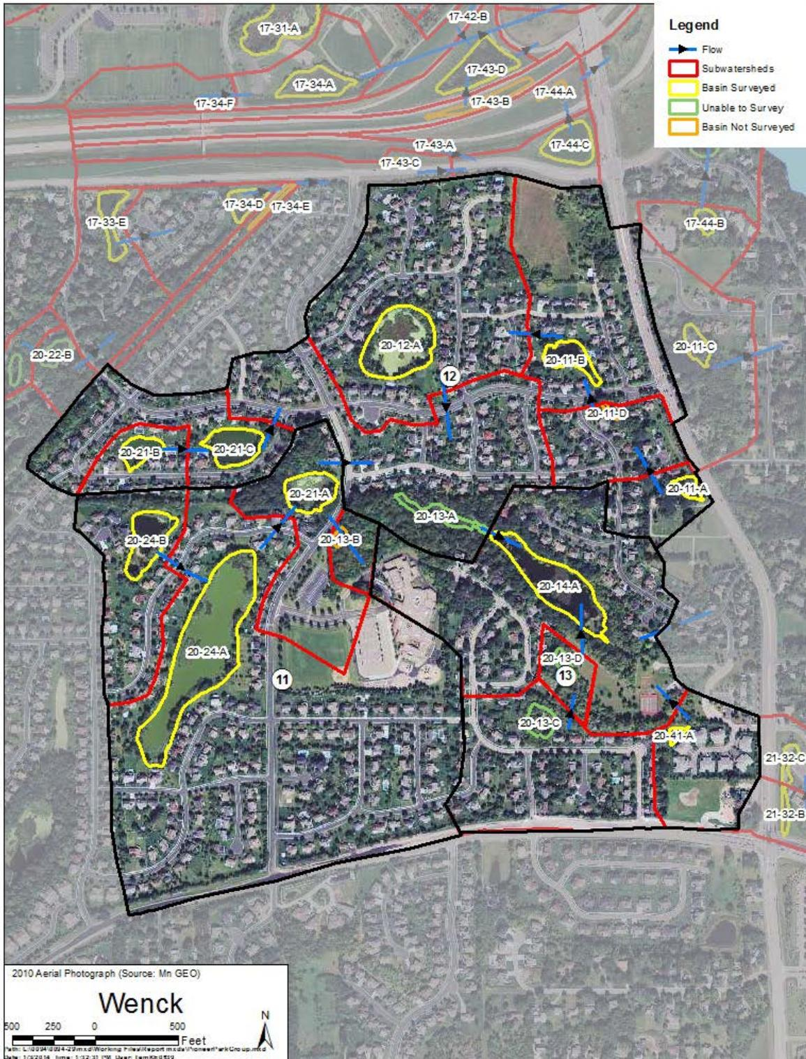
**Figure 3.8. Constructed Ponds, Wetlands and Flow Patterns in the Pioneer Creek Area Subwatershed.**
