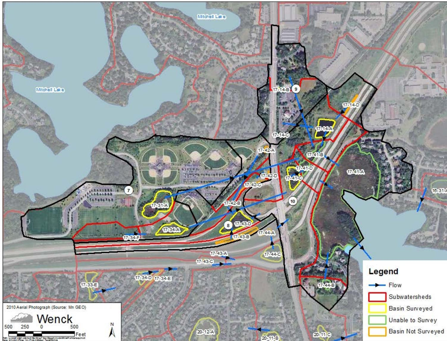
Figure 3.6. Constructed Ponds, Wetlands and Flow Patterns in the Miller Park and Highway 212 Area Subwatershed.
