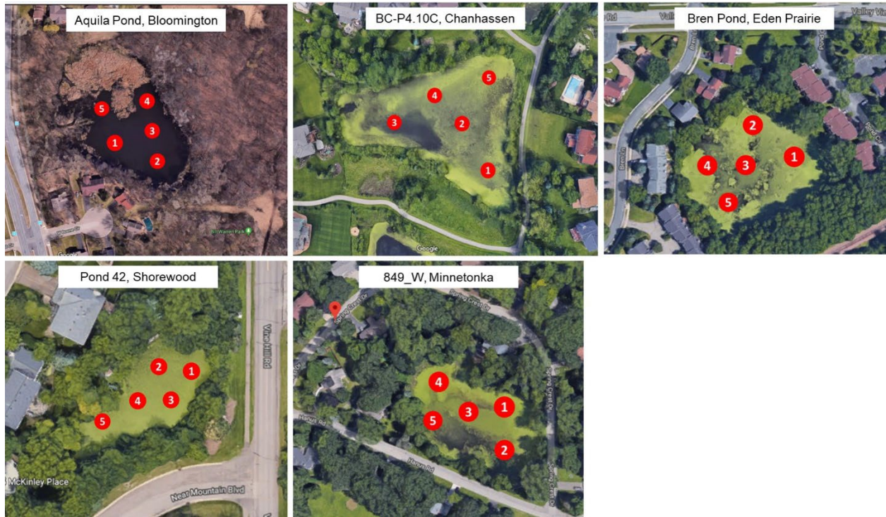
Figure A- 2. Maps showing the locations of surface water sample collection (1-5 red circles) and profile measurement (deepest location) in the RPBCWD ponds sampled from 2019-2021. Hypolimnion water samples were collected at the deepest location (typically pond center except for Aquila). Sediment cores for laboratory phosphorus release study were collected close to the marked locations.
