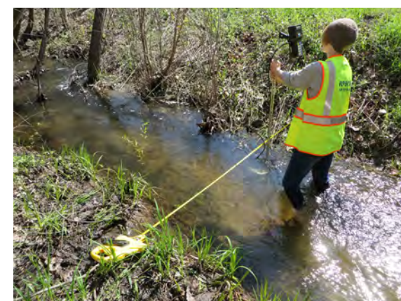
Staff measure velocities and calculate flow on Riley Creek. Measurements are conducted every two weeks from May to September at five sites.
