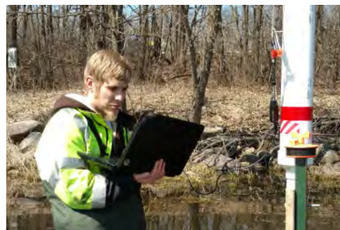
Staff checking a water level sensor on Hyland Lake. The sensor tracks how high the lake gets.
