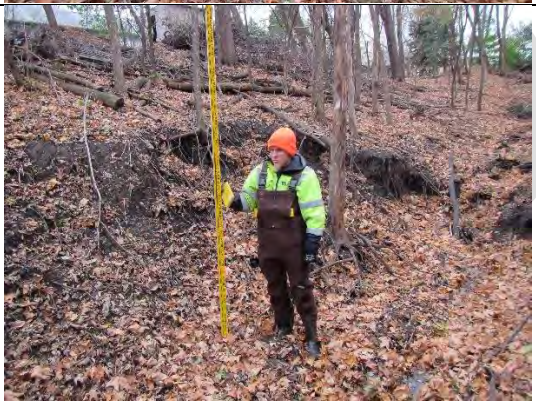
IMG_2112 Start of stream flow; erosion on RB, 3ft to 6ft high for 100yd.
