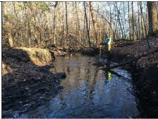
IMG-0264 Large stretch of deposition along right bank, 6m long
