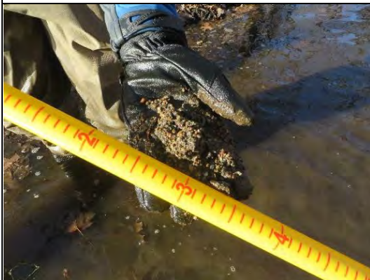
IMG-0246 Sediment is 50/50 sand/silt
