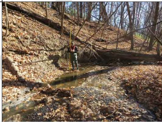
IMG-0191 Right bank erosion, 0.5m
