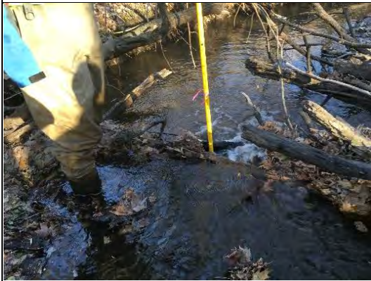
IMG-0300 Woody debris dam holding back about 0.3m of water
