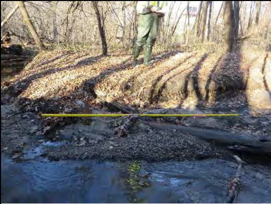
IMG-0262 Large deposition area on left bank, 3.5 m long
