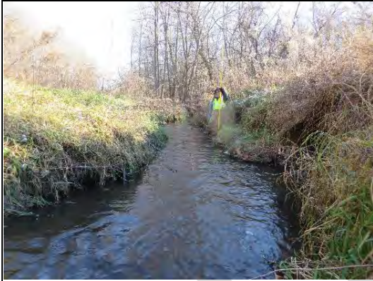
IMG-0259 Decrease in width and depth; increase in grasses; evidence of sloughing, right bank
