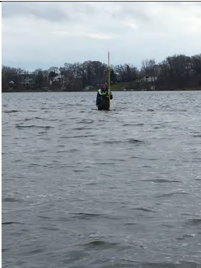
IMG-0342 Sand/silt deposition creating delta projecting about 30m into Lake Susan
