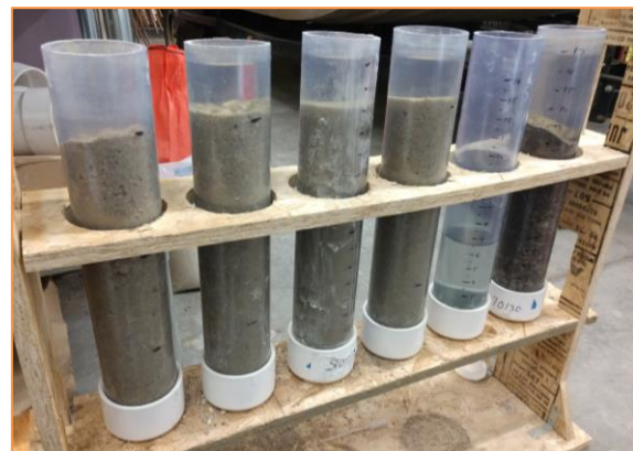
Figure 35 Spent Lime/Sand Mixture Column Testing
