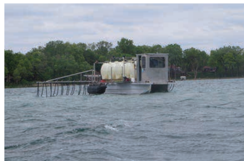
A professional crew applies Alum to Lake Riley with a specialized boat.
