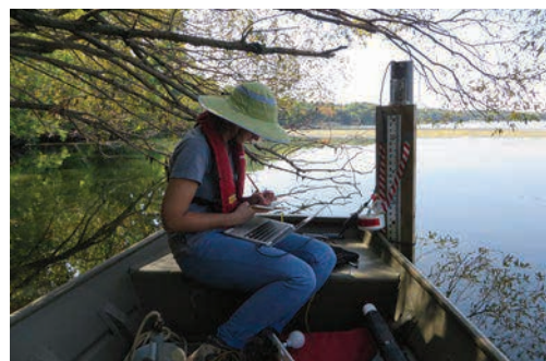
A staff member collects water level data from a sensor installed on Lake Riley. These data are available through the DNR Lake Finder Website.
