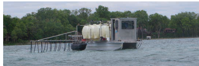
An alum barge treating a lake.
