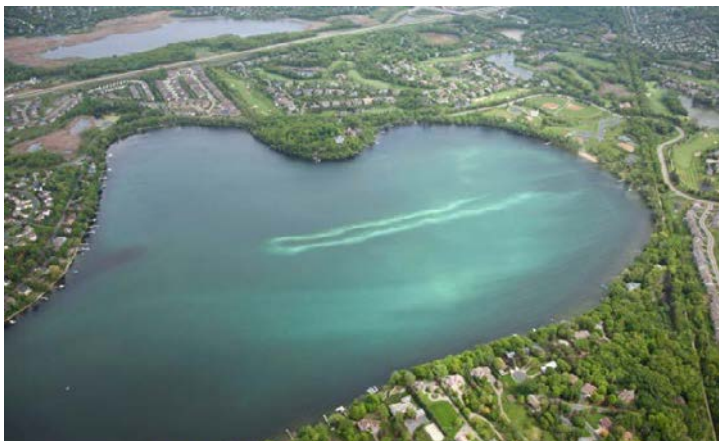
Photo: Lake Riley, after treatment with aluminum sulfate. The light blue line shows where the alum was placed.
