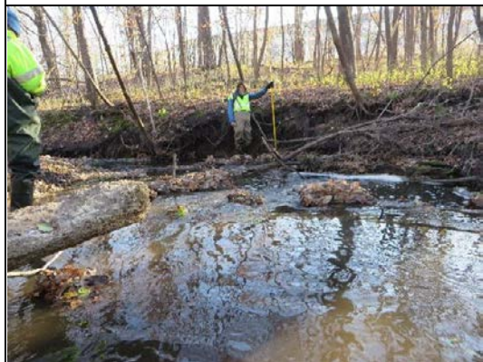
IMG-0261 Woody debris dam; erosion 1.4m x 4m long on right bank
