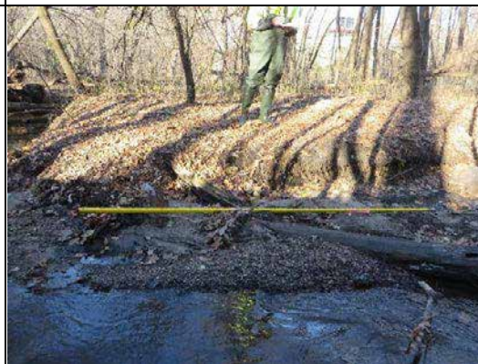
IMG-0261 Woody debris dam; erosion 1.4m x 4m long on right bank
