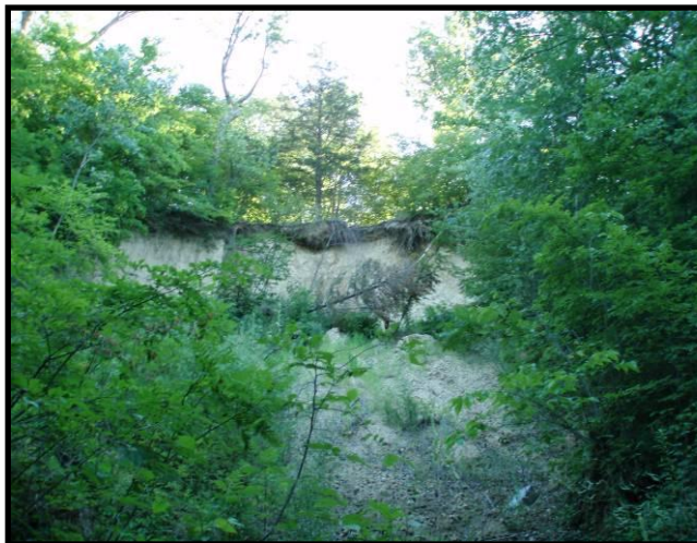
Figure 4.32 Large slope failure with wet Soils on Lower Area and dense sandy clay soils on upper bank. (Site 16)
