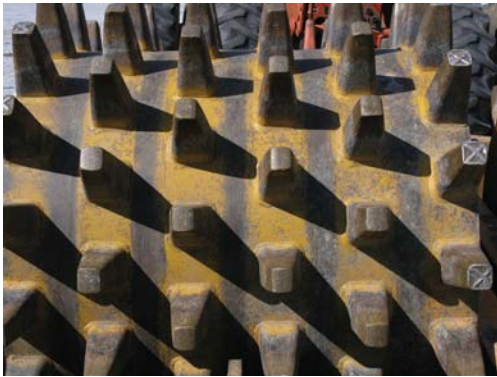
Figure 5.3: Sheepsfoot rollers compact soil.
