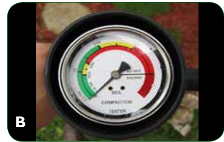
FIGURE 2.20 A and B. Measuring surface and subsurface hardness with a penetrometer.
