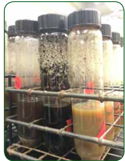
The Cornell Assessment of Soil Health identifies biological and physical soil constraints in addition to conventional soil testing. From left to right: wet aggregate stability, root pathogen pressure and soil protein tests in the lab.
