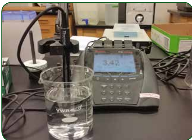
FIGURE 2.52. Electrical conductivity (EC) meter used to measure salinity.
