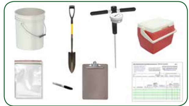
FIGURE 2.06. Materials needed to collect at least one soil health sample.
