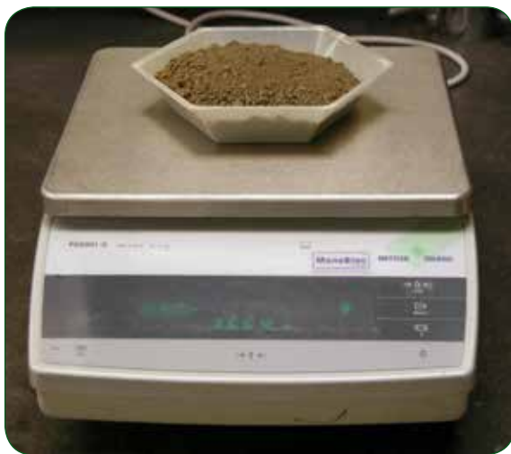
FIGURE 2.28. Soil mass is determined prior to being exposed to high temperature. Soil is weighed after being ashed to calculate the percentage of mass lost.
