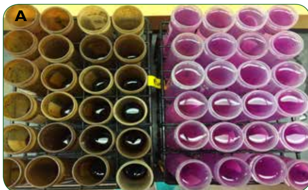
FIGURE 2.37 A and B. (A) Extracts before and after dilution. The samples on the left are after they have been weighed, shaken, and settled. The samples on the right show the dilution as they are prepared for (B) samples are measured for absorbance at 550 nm.
