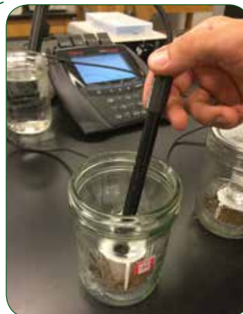
FIGURE 2.35 A-C. Soil Respiration is measured by capturing and quantifying \text{CO}_2 released from samples.
