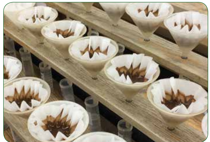
FIGURE 2.41. Potentially Mineralizable Nitrogen (PMN) processed in the lab. The difference between pre-incubation and post-incubation ammonium measurements is used as an indicator of N mineralization.
