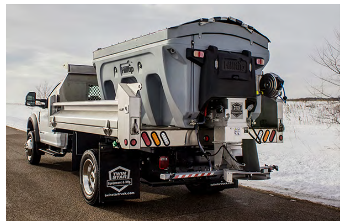
Eden Prairie Independent School District #272 used Chloride Reduction Grant Funds to replace two outdated salt spreaders with more advanced equipment that can be calibrated to conditions and ultimately reduce salt use.
